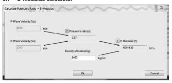
Enter the P- and S-wave pulse velocities to calculate the Poisson's ratio. Additionally enter the density of the material to calculate the E-modulus.
