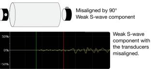
Rotate one transducer into and out of alignment and watch the S-wave component increase and decrease.
